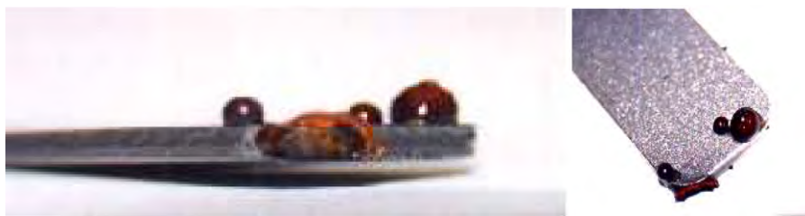
Fig. 3.11 Corrosion “balls” formed on a carbon steel surface (strip coupons) after 3 days’ immersion in kerosene with water (1 wt %) added.
