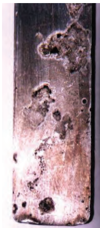
Fig. 2.4 Under deposit corrosion : corrosion pits formed under \text{NH}_4\text{Cl} acidic salt deposits on a carbon steel surface (4 months).
