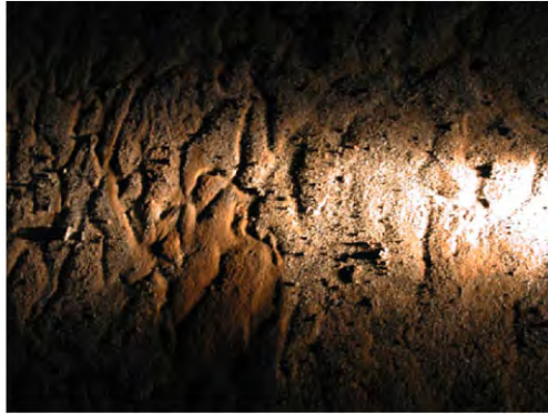
Fig. 3.17 Corroded bottom of a crude oil AST. The morphology of the surface and microbiological examination showed MIC.
