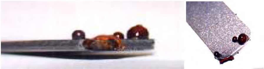
Fig. 3.11 Corrosion “balls” formed on a carbon steel surface (strip coupons) after 3 days’ immersion in kerosene with water (1 wt %) added. (For a full color version of this figure, see the Color Section)
