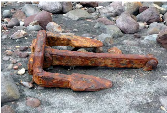
Fig. 1.12 Corroded anchor made of carbon steel.
