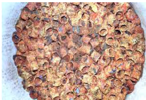
Fig. 6.6 Beauty of corroded Raschig rings in an oil refinery. (For a full color version of this figure, see the Color Section)
