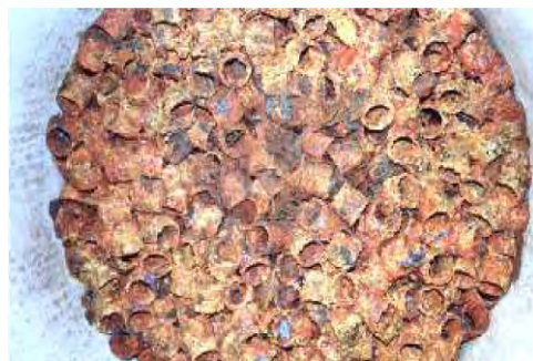
Fig. 6.6 Beauty of corroded Raschig rings in an oil refinery.
