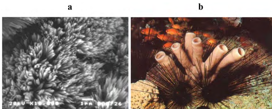
Fig. 6.19 (a) SEM photo ( \times 10,000 ) of rust formed in the heat exchanger of a overhead crude distillation column; (b) black sea urchins.
