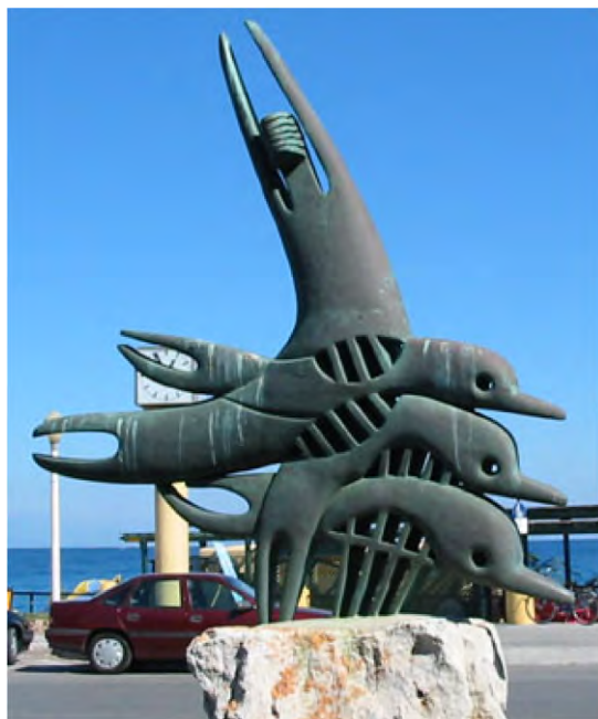
Fig. 3.5 Natural patina formed on a bronze statue. (For a full color version of this figure, see the Color Section)
