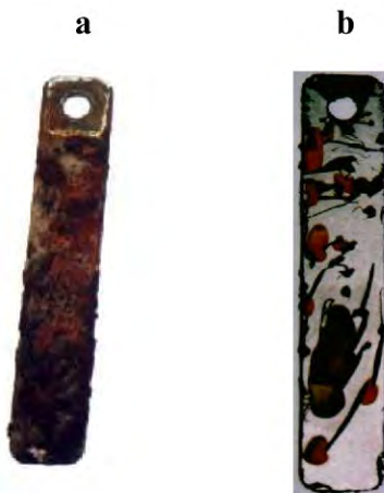
Fig. 1.17 Carbon steel after 7 days immersion in cooling water (a) and in water with the addition of sodium peroxoborate ( \text{NaBO}_3 ) (b). The “beautiful” rust is formed on the steel’s surface in a \text{NaBO}_3 solution.
