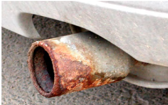
Fig. 3.8 The exhaust system of a vehicle after dewpoint corrosion. (For a full color version of this figure, see the Color Section)
