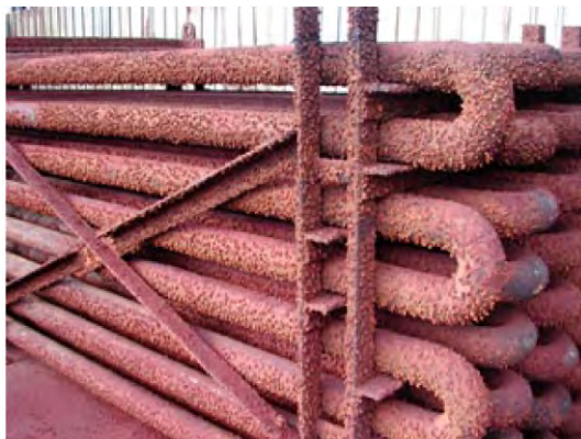
Fig. 3.1 Carbon steel tubes used in contact with water. (For a full color version of this figure, see the Color Section)
