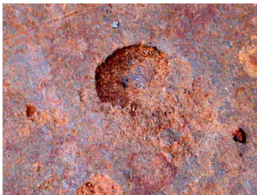
Fig. 2.10 MIC on a metal surface compared with pitting, crevice, differential aeration cell, or galvanic corrosion. The bottom of a crude oil storage tank after a microbial attack.
