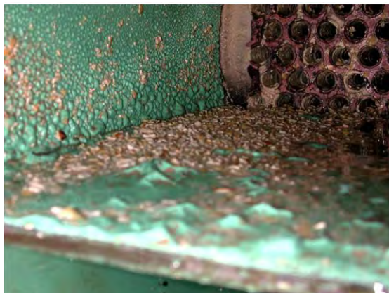
Fig. 3.2 Scale (calcium and magnesium carbonates) formed inside of heat exchanger with cooling water after 4 years.
