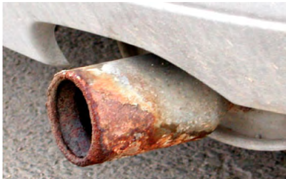
Fig. 3.8 The exhaust system of a vehicle after dewpoint corrosion.
