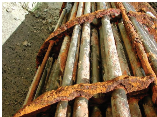
Fig. 2.6 Heat exchanger: tubes made of titanium and baffles made of carbon steel (cooling water, 4 years). Deposits on the titanium tubes are the salts (scale) formed from the cooling water, and not corrosion products.
