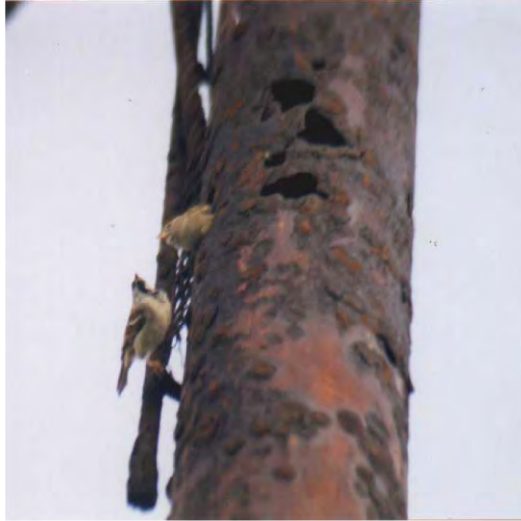
Fig. 6.24 “Corrosion led to contentment”. Corroded mast of a ship (Haifa Bay).
