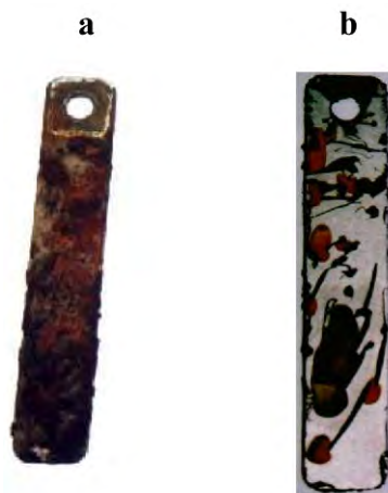
Fig. 1.17 Carbon steel after 7 days immersion in cooling water (a) and in water with the addition of sodium peroxocarbonate ( \text{NaBO}_3 ) (b). The “beautiful” rust is formed on the steel’s surface in a peroxocarbonate solution. (For a full color version of this figure, see the Color Section)
